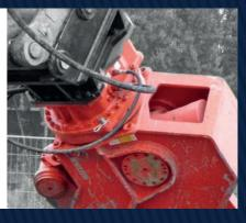
The speed valve developed by Rotar allows the jaws to close quickly and automatically switch from speed to power mode as soon as the job requires
